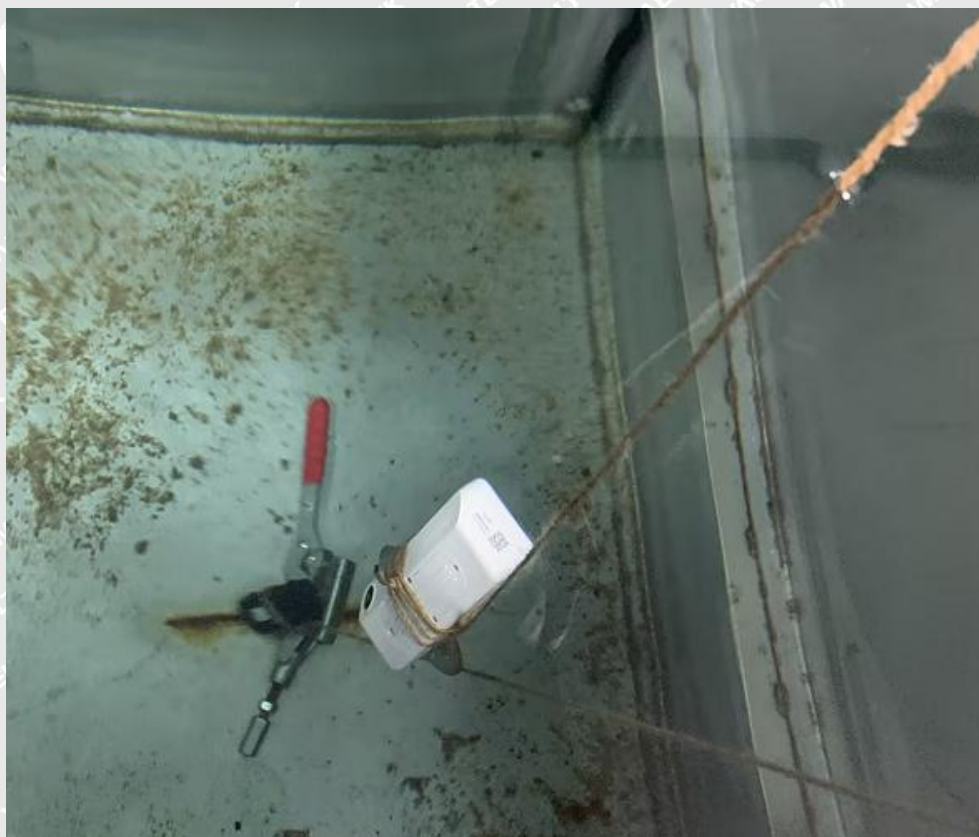
During the IP X7 test
