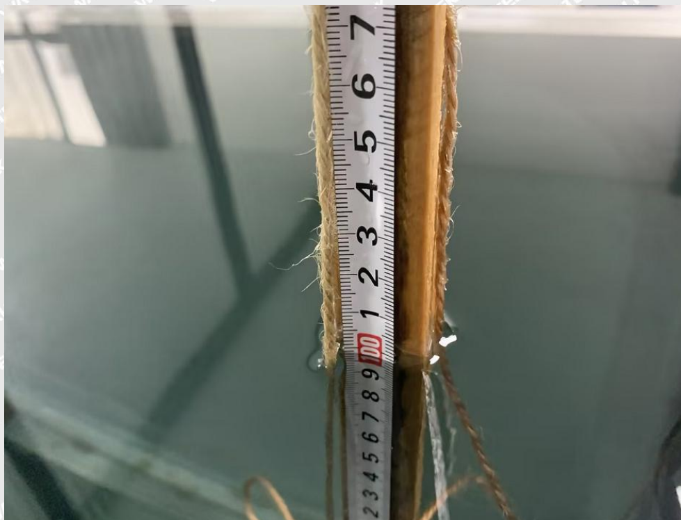
IP X7 water height 1m
